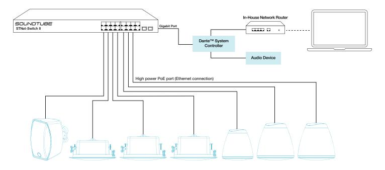
IPD speakers connect to the Dante network via a PoE switch such as the SoundTube STNet Switch II. All setup is done centrally; speakers are self monitoring and will report any issues back to the management software, meaning one glance will tell you if the system is working properly. For economical system expansion, IPD4 speakers provide audio and power to standard (non-Dante) CM-BGM speakers.
